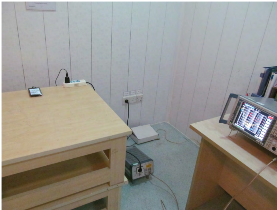
FCC LINE CONDUCTED EMISSION TEST SETUP
