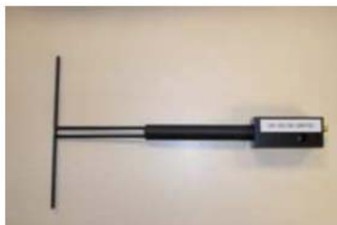
Figure 1 – Satimo COMOSAR Validation Dipole
