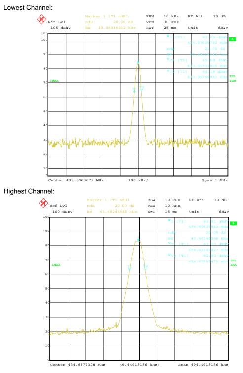
The results: The unit does meet the FCC Part 15 C Section 15.231 requirements.
