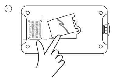
Remove the battery from the bottom of the joystick.
