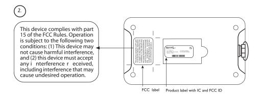
The FCC statement is placed to the left. The product label is placed behind the battery in the battery compartment on the bottom of the joystick transmitter.
