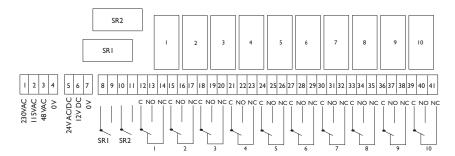
**IMPORTANT!** To utilize the safety, relays **SR1** and **SR2** shall be used as stop relays in the safety circuitry of the object to be controlled.
