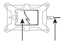
BATTERY TYPE: CHARGE: CHARGING TEMPERATURE: OPERATING TIME: External and rechargeable lithium-ion In the charger unit 5V DC ±10% (1A) 0°C to 45°C/ 32°F to 113° Approx. 15 h. with continuous usage
