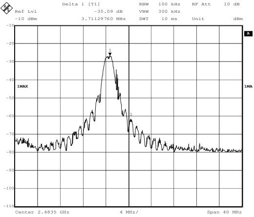
For 2483.5MHz bandedge checked with 2480MHz frequency operated, the delta shown at the plots are 35.09dB for peak detector mode.
