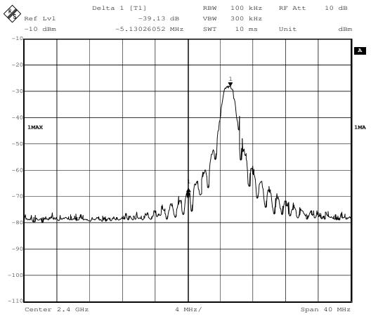
For 2400MHz bandedge checked with 2405MHz frequency operated, the delta shown at the plots are 39.13dB for peak detector mode.
