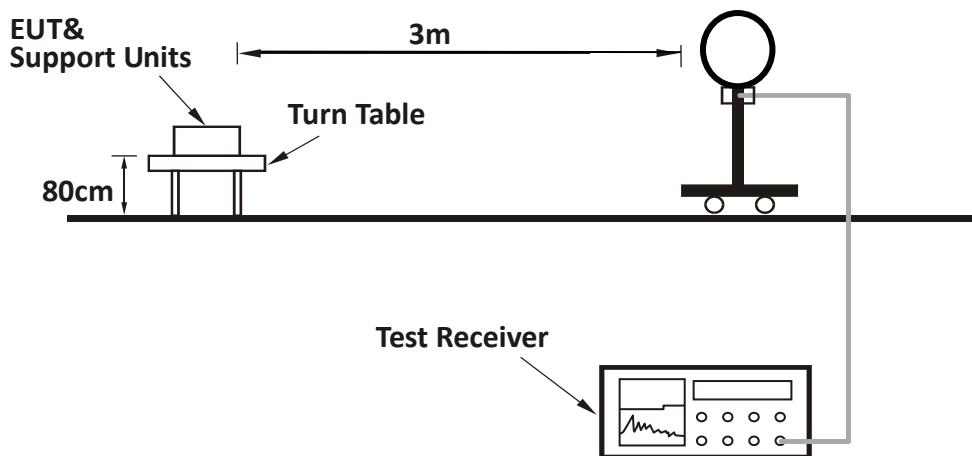
For Radiated emission 30MHz to 1GHz:
