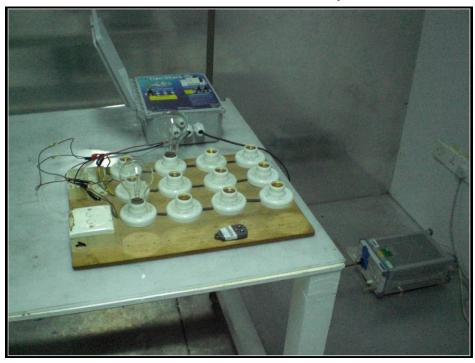
Radiated Emissions, 30MHz to 1GHz Test Setup
