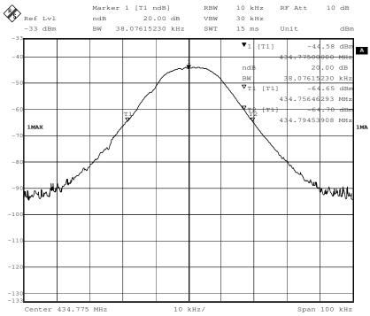
The results: The unit does meet the FCC Part 15 C Section 15.231 requirements.
