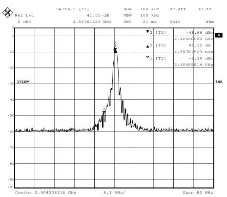
For 2.40GHz band edge checked with 2.405GHz frequency operated, the delta shown at the plots are 41.35dB for peak detector mode.
