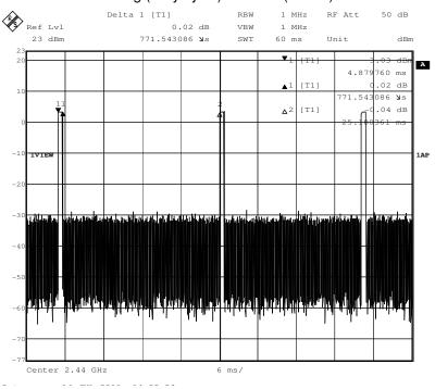
Middle channel: 20log (Duty cycle)=20\*log(0.891703557/25.1800361)=-29.02dB; Vertical: Average = Peak value + 20log (Duty cycle)= 92.09+(-29.02)=63.07dBuV/m Horizontal: Average = Peak value + 20log (Duty cycle)=89.75+(-29.02)=60.73dBuV/m
