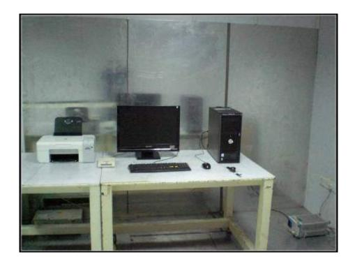
Radiated Emissions, 30MHz to 1GHz Test Setup
