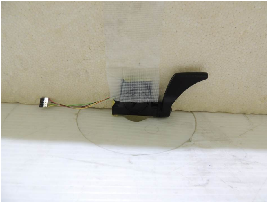
Photograph 5: Set-up for Radiated Emission, EUT Configuration Y-Axis
