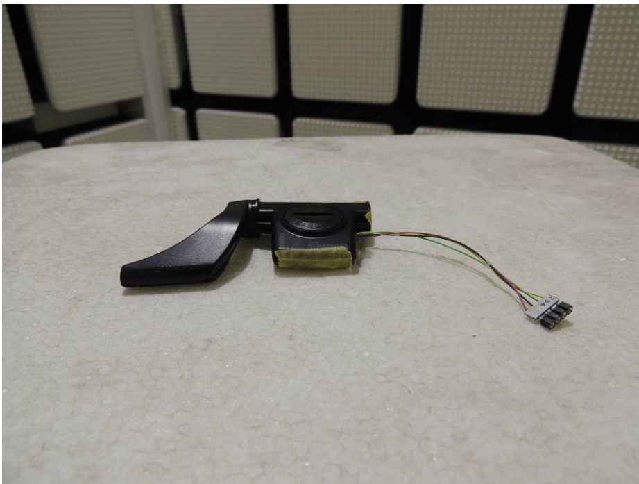
Photograph 4: Set-up for Radiated Emission, EUT Configuration X-Axis
