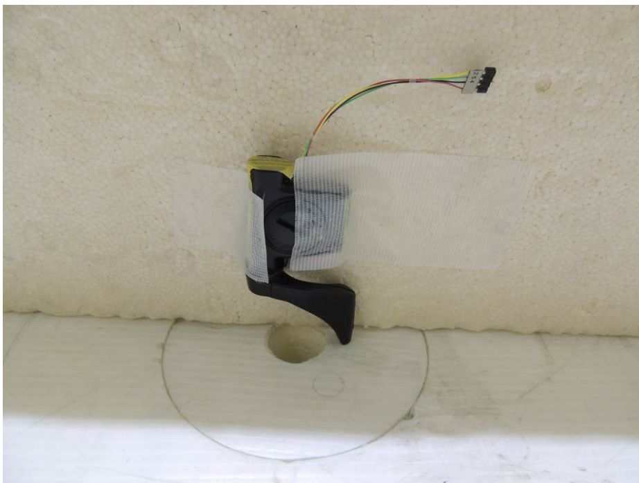
Photograph 6: Set-up for Radiated Emission, EUT Configuration Z-Axis
