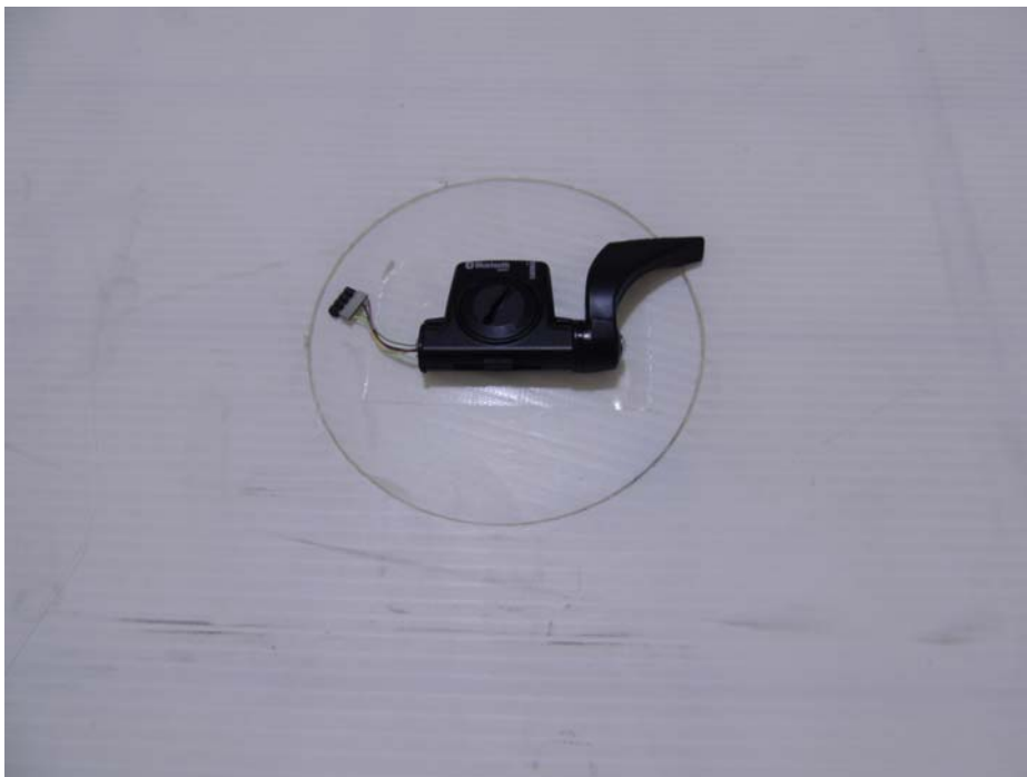
Photograph 5: Set-up for Radiated Emission, EUT Configuration X-Axis
