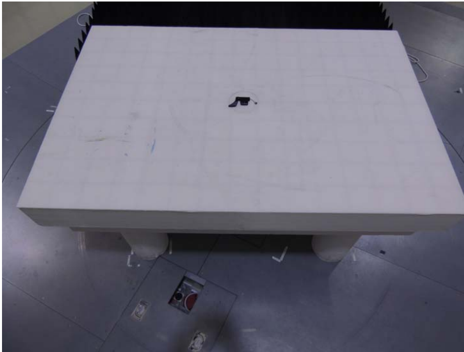
Photograph 4: Set-up for Radiated Test of Transmitter, Rear View
