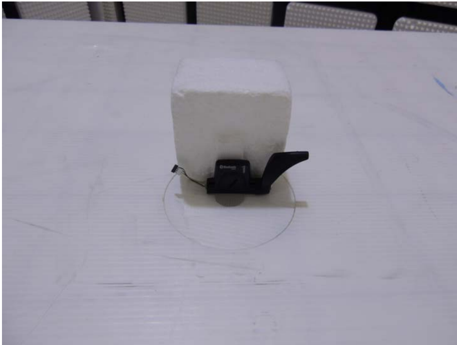
Photograph 6: Set-up for Radiated Emission, EUT Configuration Y-Axis
