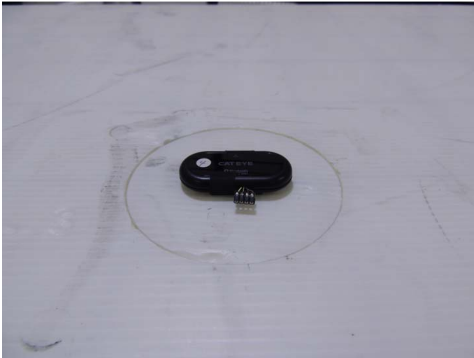
Photograph 4: Set-up for Radiated Emission, EUT Configuration X-Axis
