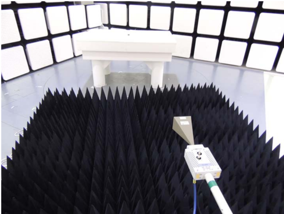
Photograph 3: Set-up for Radiated Emission of Transmitter, Measuring Antenna View
