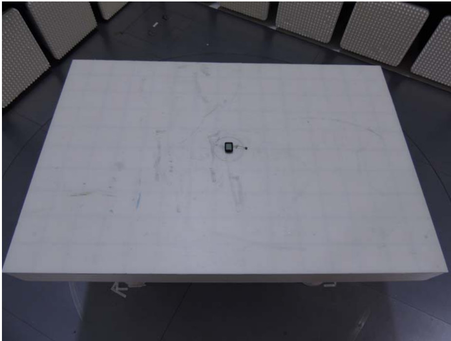
Photograph 2: Set-up for Radiated Test of Transmitter, Table View
