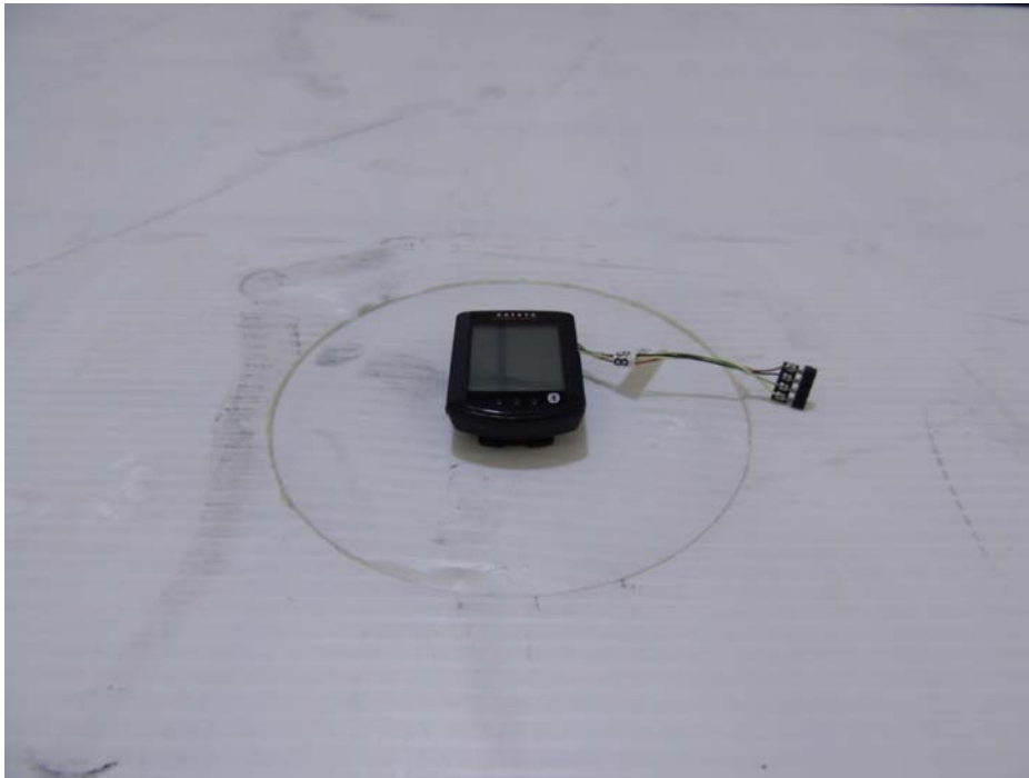
Photograph 4: Set-up for Radiated Emission, EUT Configuration X-Axis
