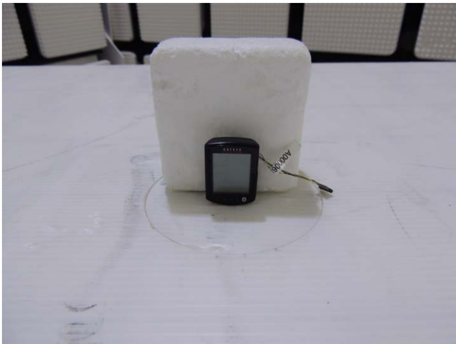
Photograph 5: Set-up for Radiated Emission, EUT Configuration Y-Axis
