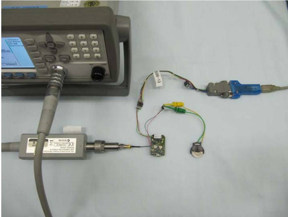
Photograph 1: Set-up for RF Conducted Power at Antenna Port
