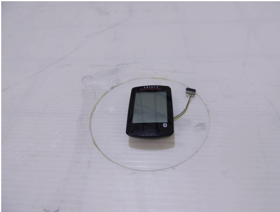
Photograph 4: Set-up for Radiated Emission, EUT Configuration X-Axis at 80cm height
