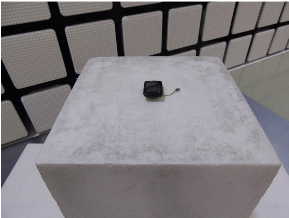
Photograph 7: Set-up for Radiated Emission, EUT Configuration X-Axis at 1.5m height
