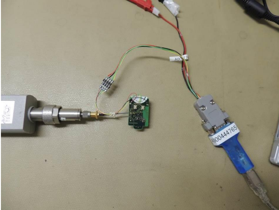
Photograph 1: Set-up for Conducted Emissions at Antenna Port
