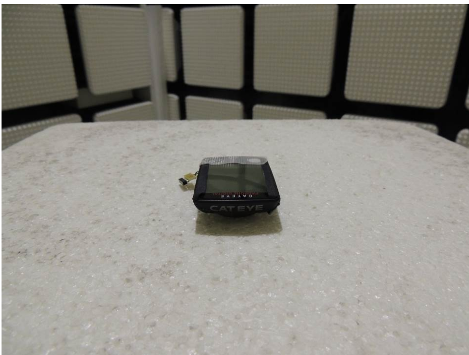
Photograph 4: Set-up for Radiated Emission, EUT Configuration X-Axis
