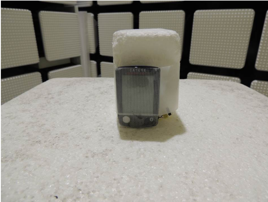
Photograph 5: Set-up for Radiated Emission, EUT Configuration Y-Axis
