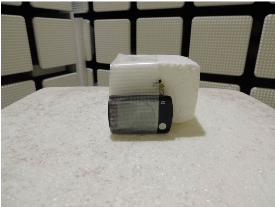
Photograph 6: Set-up for Radiated Emission, EUT Configuration Z-Axis
