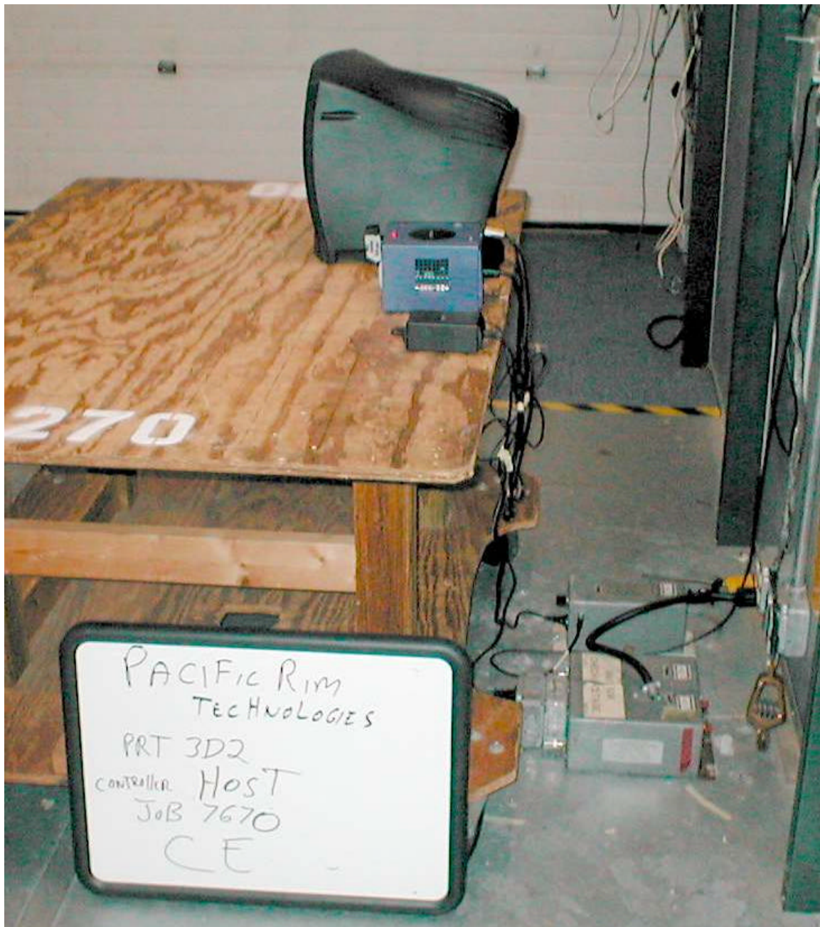
Conducted Spurious Emissions Test Setup, Side
