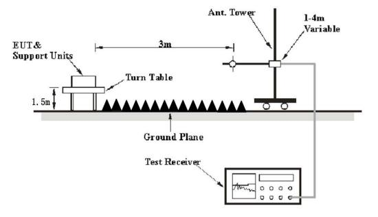
The radiated emission tests were performed in the 3 meters test site, using the setup accordance with the ANSI C63.10 - 2013. The specification used was the FCC 15  $\S$  15.209, 15.205 and 15.231.
