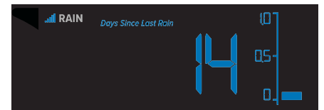
Up to 1" Example Each Segment Equals 0.1" Over 1" Example Each Segment Equals 0.4"
