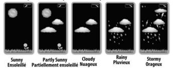
The forecast station samples the barometric pressure every twelve minutes. These samples are averaged hourly and daily then stored in nonvolatile memory.
