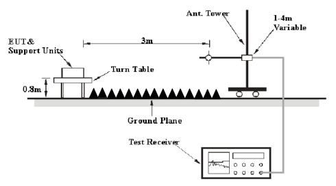
The radiated emission tests were performed in the 3 meters test site, using the setup accordance with the ANSI C63.4 - 2003. The specification used was the FCC 15 § 15.209, 15.205 and 15.231.
