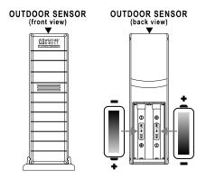
The Outdoor Temperature Sensor uses 2 x "AA", **Alkaline** batteries. To install and replace the batteries, please follow the steps below:
