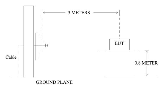
(EUT: Temperature transmitter)
