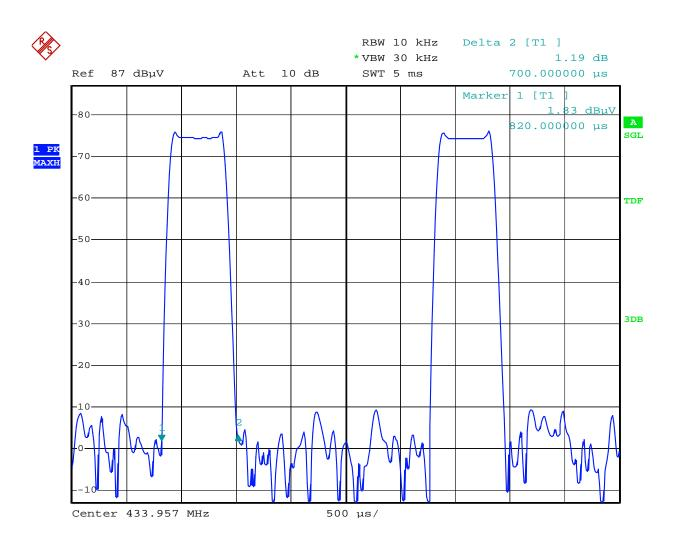
The graph shows the duration of 'on' signal. From marker 1 to marker 2, duration is 0.7 ms.
