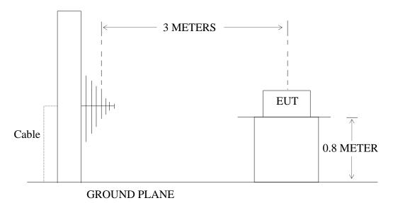
(EUT: Temperature transmitter)
