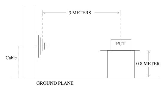
(EUT: Temperature transmitter)
