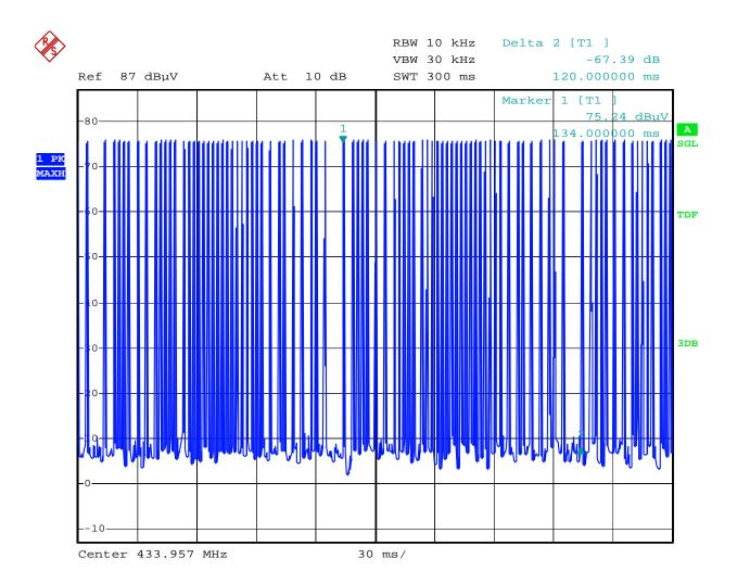
The duration of one cycle is 120 ms; it shows 37 'on' signals.
