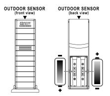
The Optional Outdoor Temperature Sensor uses 2 x "AA", **Alkaline** batteries. To install and replace the batteries, please follow the steps below:
