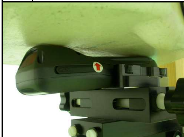
C: The bottom of the EUT face to the phantom with 0mm-separation distance.
