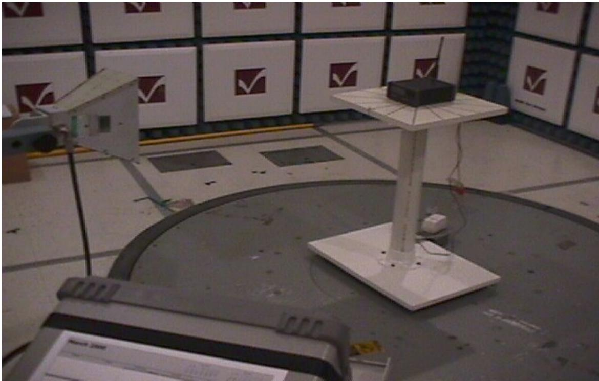
View of the QP-100 during the Conducted Emissions tests.
