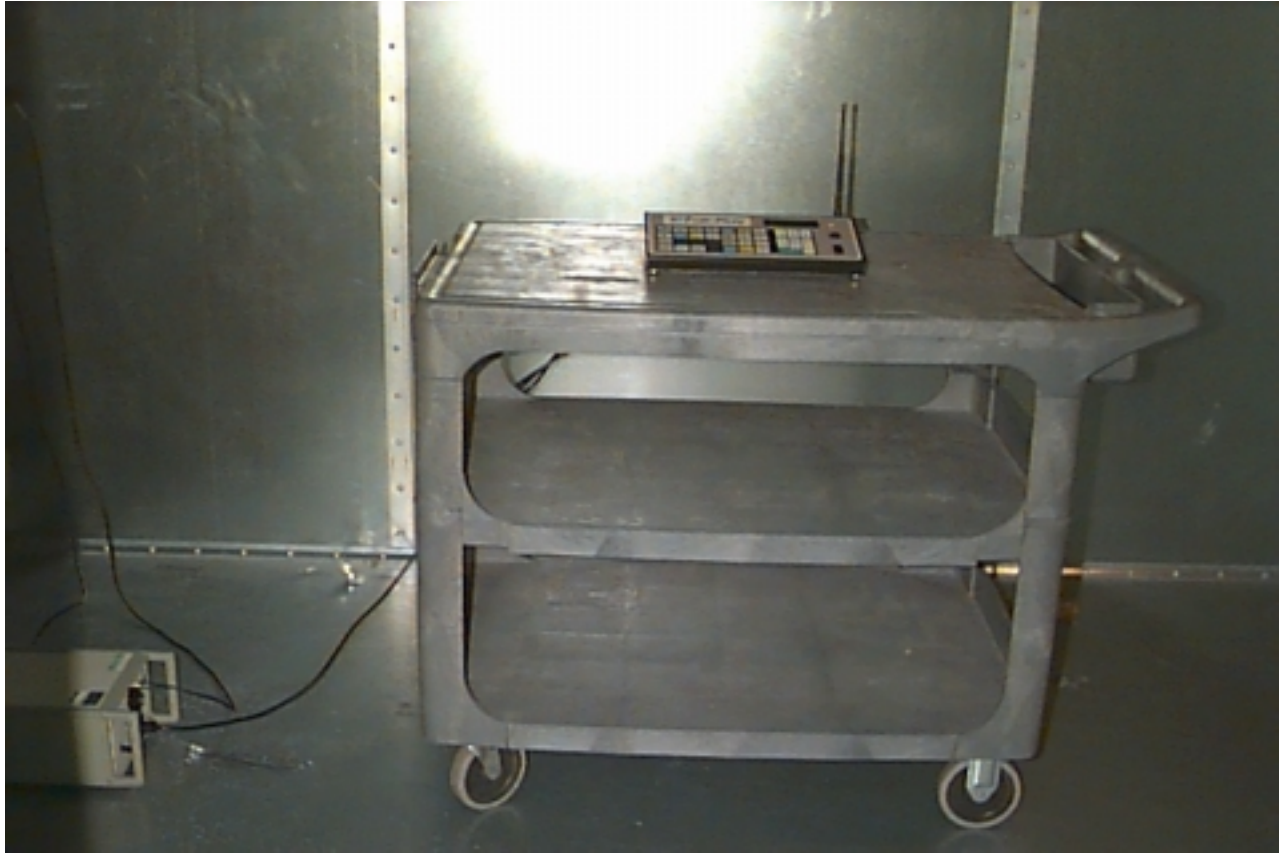
View of the Fairplay MP-70 during conducted emission testing.
