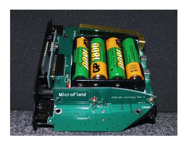
EUT: MSF0001 FM Transmitter/Receiver Receiver Antenna (72 MHz and 216 MHz) Daughter PCB side 1
