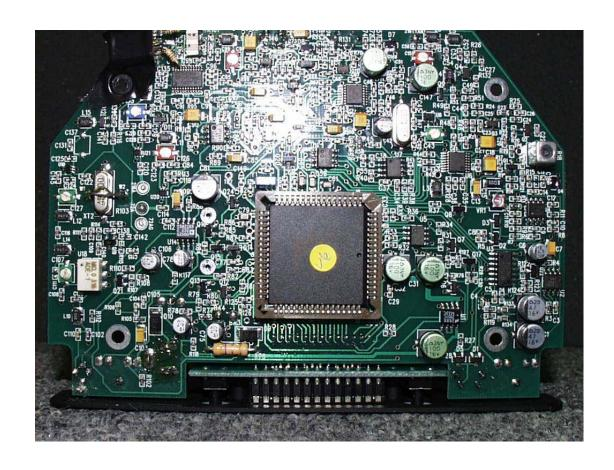
EUT: MSF0001 FM Transmitter/Receiver PCB Component side view
