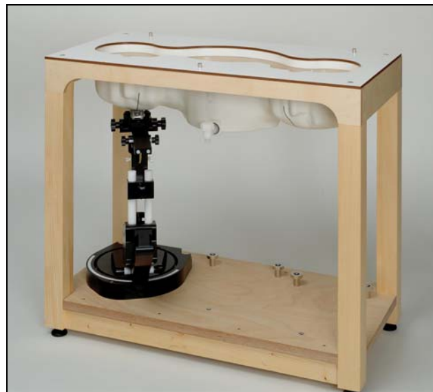
Figure 13: Specific anthropomorphic mannequin twin phantom
