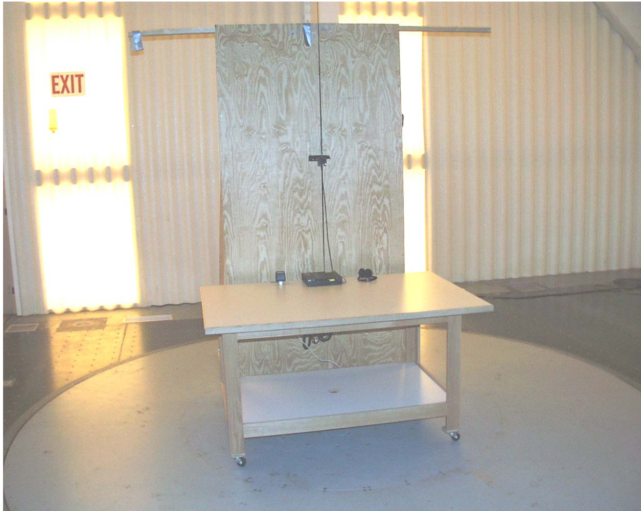
Photograph 1 - Front View Worst-Case Radiated Emission Configuration
