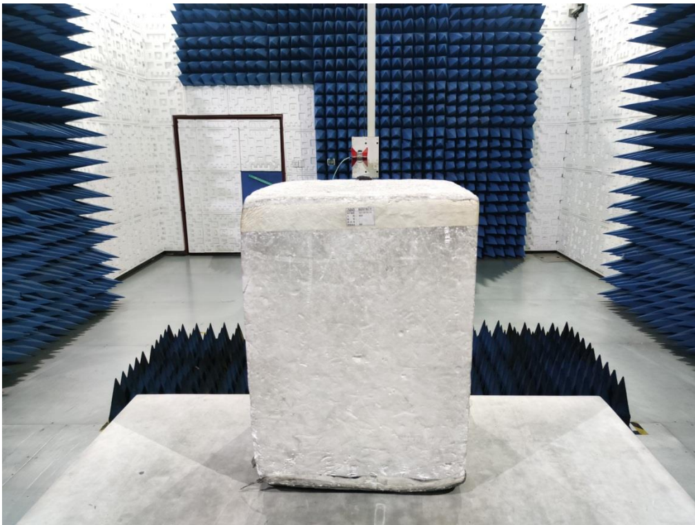
RADIATED EMISSION TEST SETUP ABOVE 1GHZ
