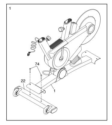
2. While a second person lifts the rear of the Base (1), attach the Rear Stabilizer (23) to the Base with two 3/8" x 2 1/4" Screws (74).
