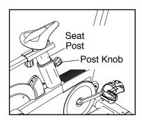
firmly tighten the post knob. Make sure that the post knob is engaged in an adjustment hole.
