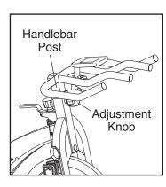
ment knob. Make sure that the adjustment knob is engaged in an adjustment hole.
