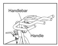
Note: The handle functions like a ratchet. To loosen the handle, turn the handle counterclockwise, pull the handle outward, turn the handle clockwise, push the handle inward, and then turn the handle counterclockwise again. Reverse this process to tighten the handle.
