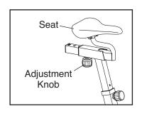
the seat carriage, and firmly tighten the adjustment knob. Make sure that the adjustment knob is engaged in an adjustment hole.
