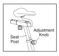
firmly tighten the adjustment knob. Make sure that the adjustment knob is engaged in an adjustment hole.
