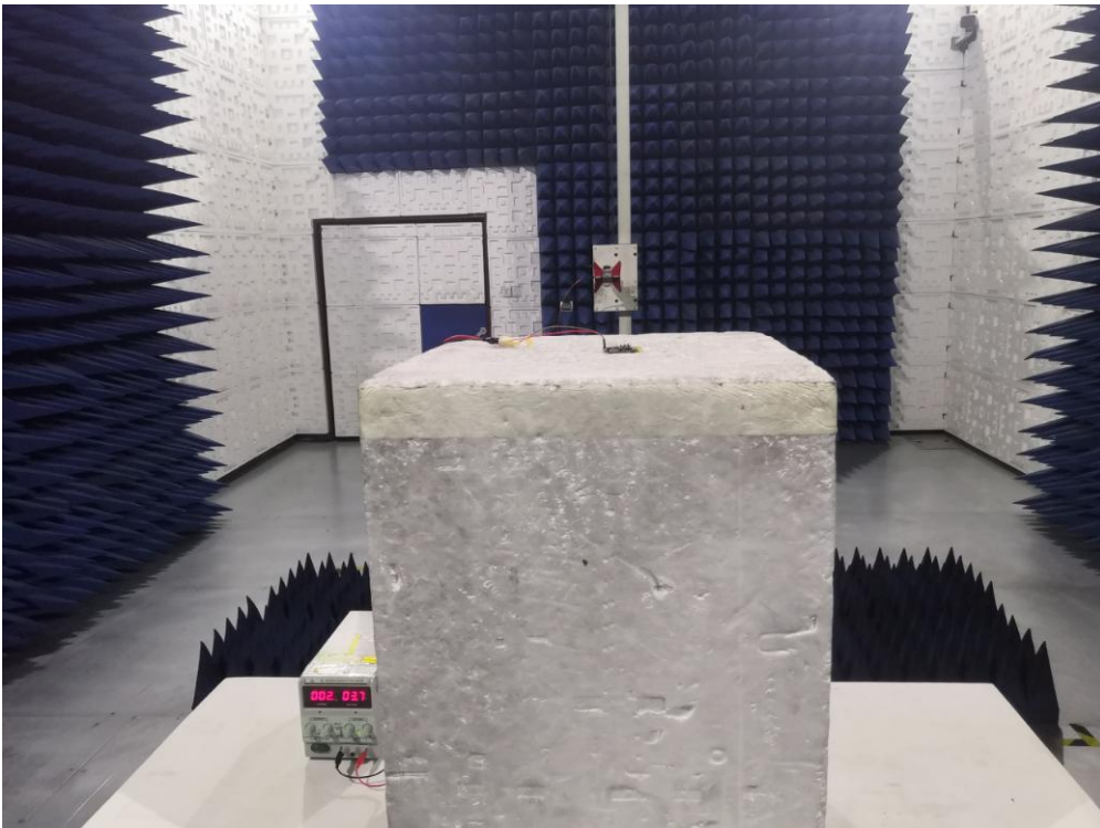
RADIATED EMISSION TEST SETUP ABOVE 1GHz
