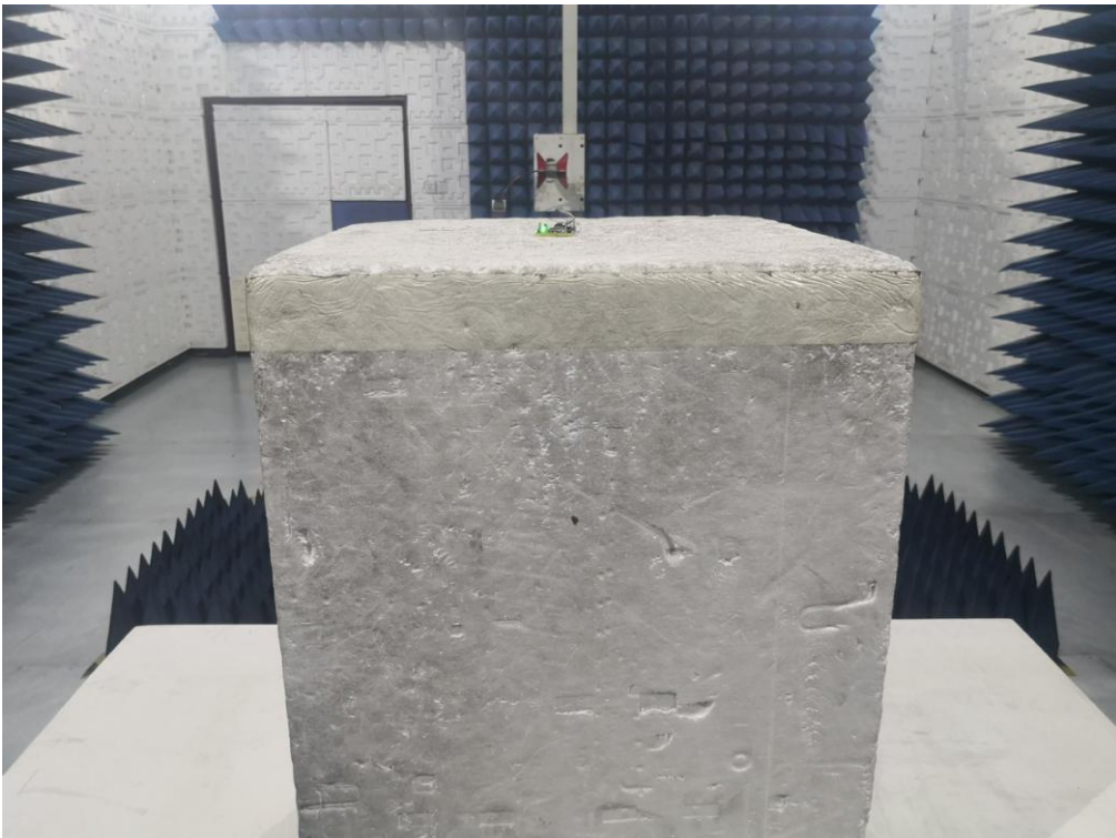
RADIATED EMISSION TEST SETUP ABOVE 1GHz
