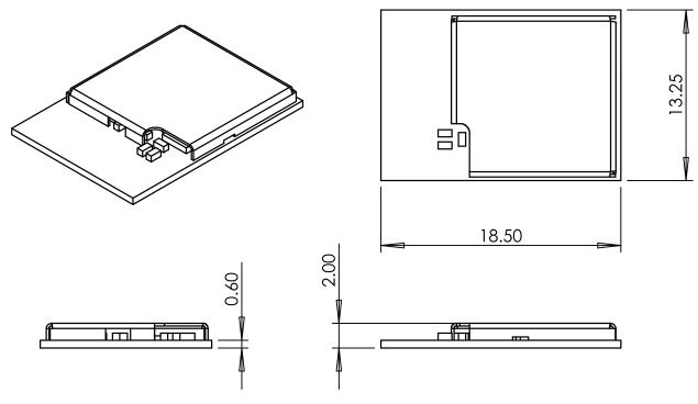
Figure 2- Module Dimensions
