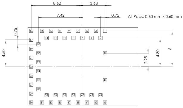
Figure 3- Module Dimensions
