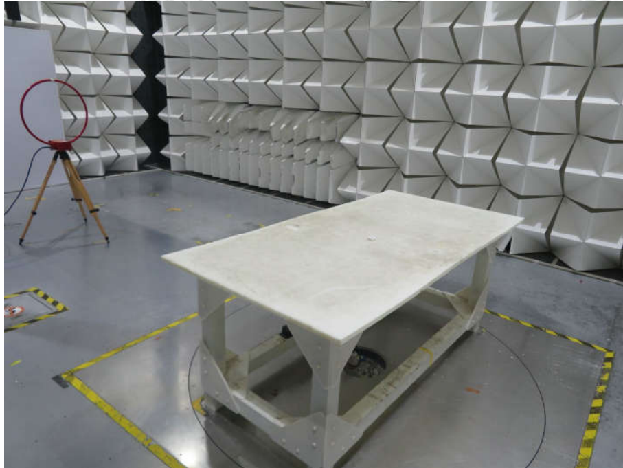
Radiated spurious emission Test Setup-1(9kHz-30MHz)
