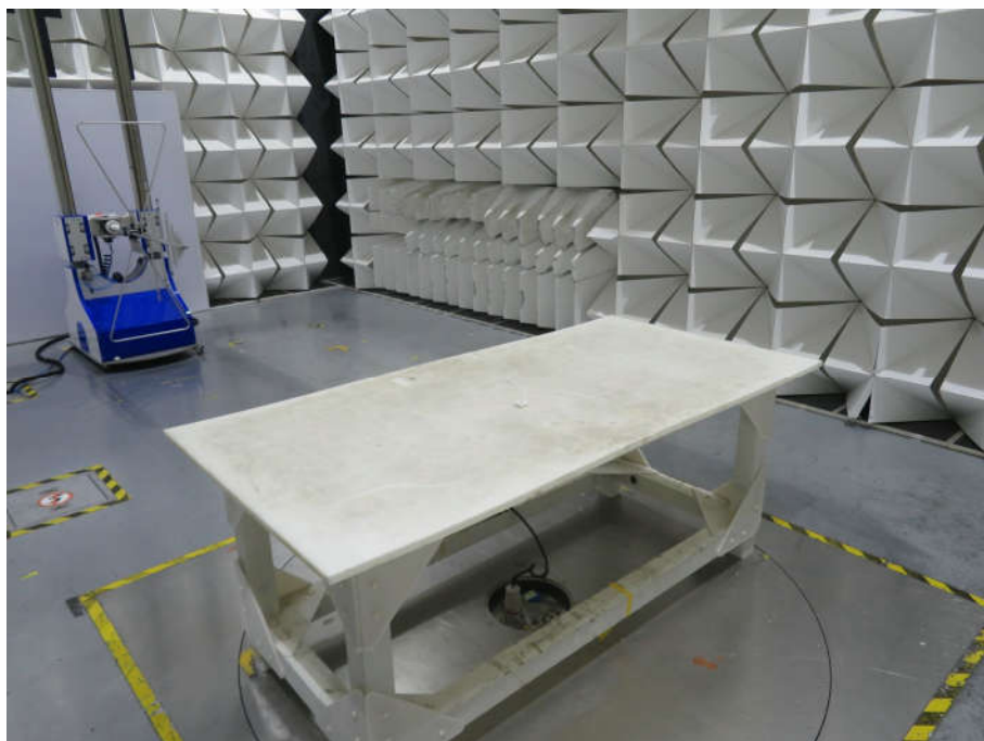
Radiated spurious emission Test Setup-2(Below 1GHz)
