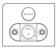
of the sensor. Insert the edge of a coin into the slot in the battery cover, turn the battery cover counterclockwise, and remove the battery cover. Next, remove the old battery and insert a new CR 2032 battery; make sure that the battery is oriented so that the text is facing away from the sensor. Then, reattach the battery cover and turn it clockwise.
