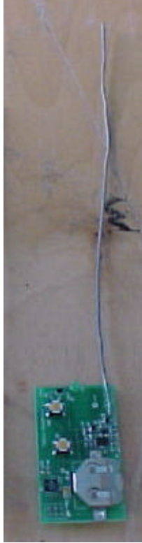
Figure 4 - Top Side of 433.92 MHz Transmitter (EUT)
