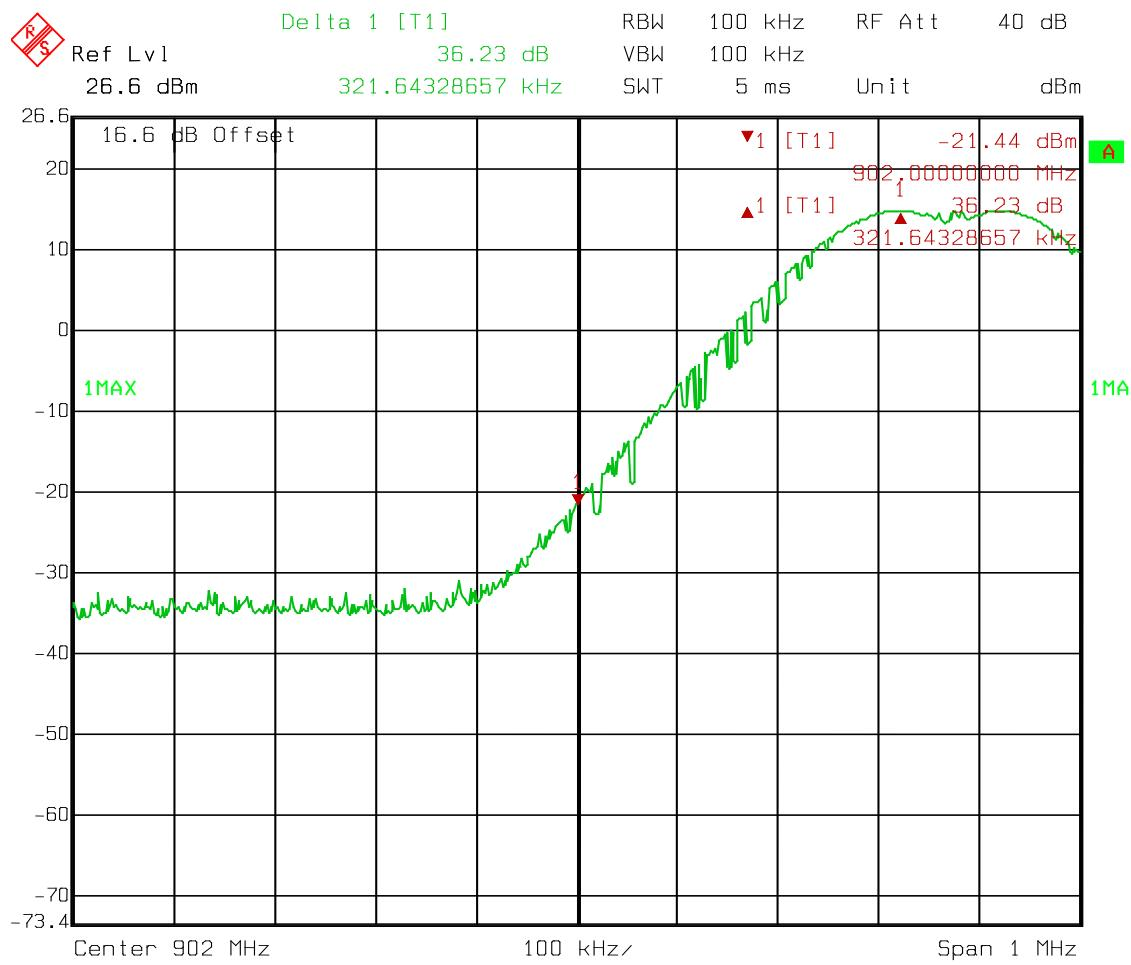
**Test Data – Spurious Emissions at Antenna Terminals****Upper Band Edge**
