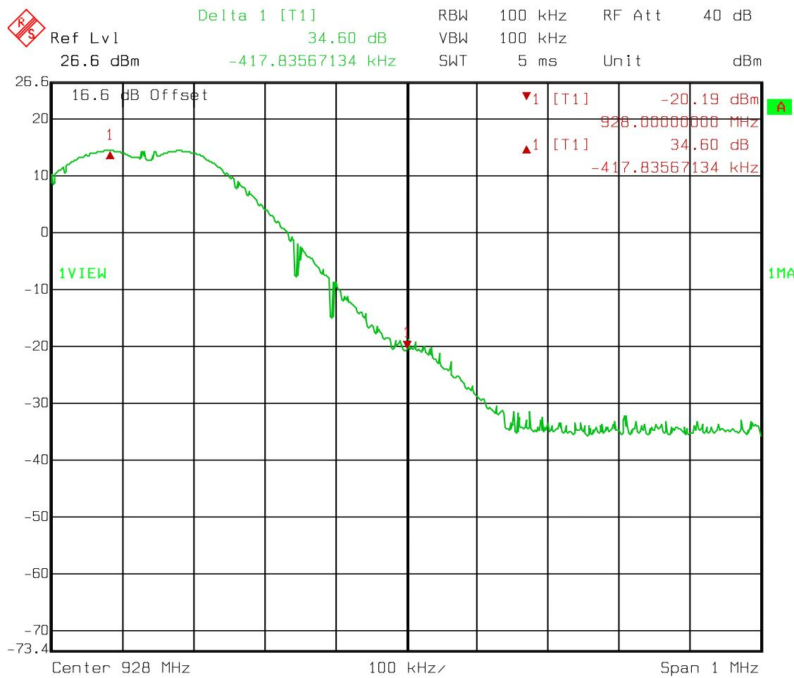
**Test Data – Spurious Emissions at Antenna Terminals**
