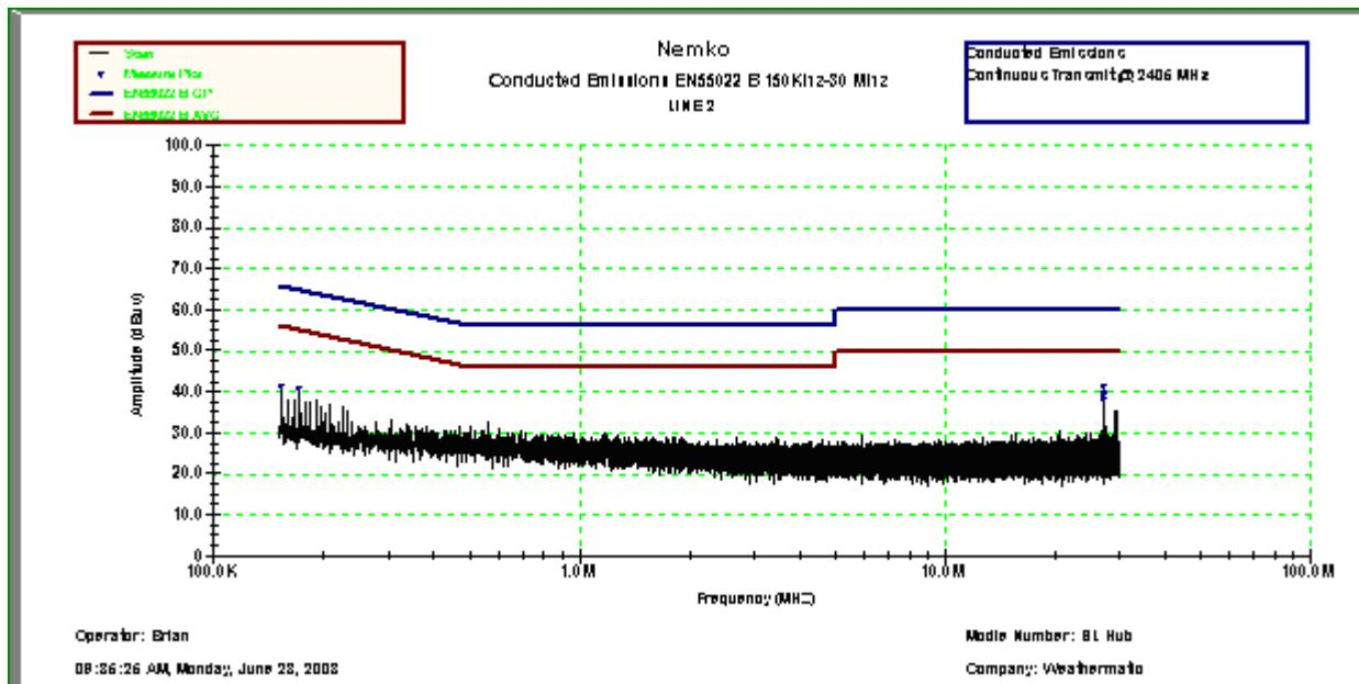
**Test Data – Powerline Conducted Emissions**
