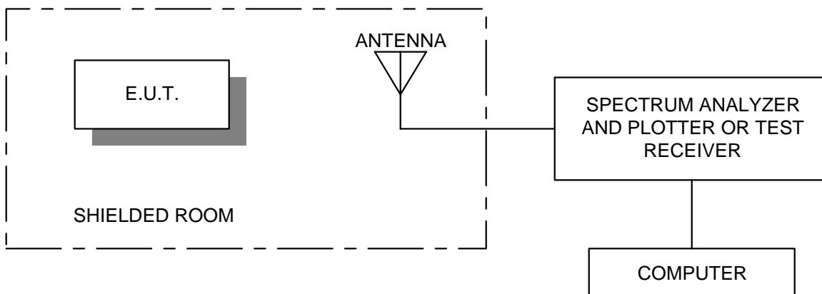
**Test Site For Radiated Emissions**
