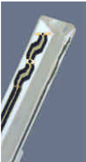
Figure 3.2 Probe Thick-Film Technique
