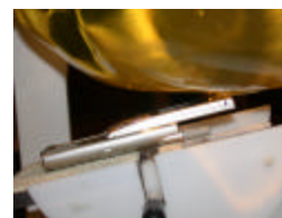
Figure A.8 Left Head SAR Test Setup -- Ear / 15° Tilt Position – (Slider Out)
