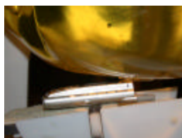
Figure A.7 Left Head SAR Test Setup -- Ear / 15° Tilt Position – (Slider In)
