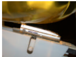
Figure A.3 Right Head SAR Test Setup -- Ear / 15° Tilt Position – (Slider In)
