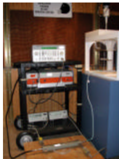
Figure A.0 Dipole Validation Test Setup
