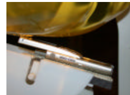
Figure A.4 Right Head SAR Test Setup -- Ear / 15° Tilt Position – (Slider Out)
