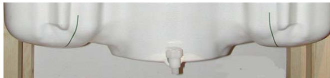
Figure 7.2 SAM Twin Phantom shell
