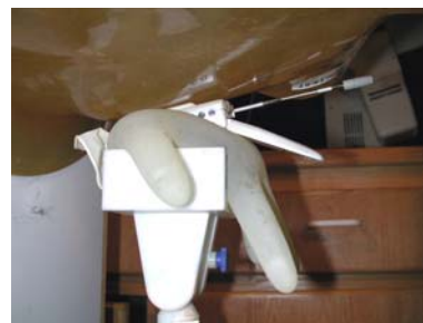
Fig. 16 Hand SAR Test Setup
