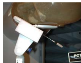
Fig. 14 Head SAR Test Setup
