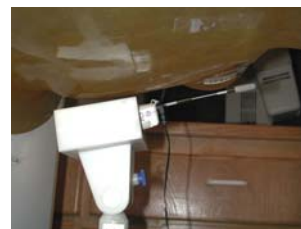
Fig. 15 Body SAR Test Setup
