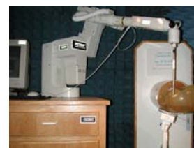
Fig. 1 SAR Test Setup
