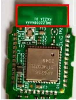
Mainboard Antenna area should be empty
