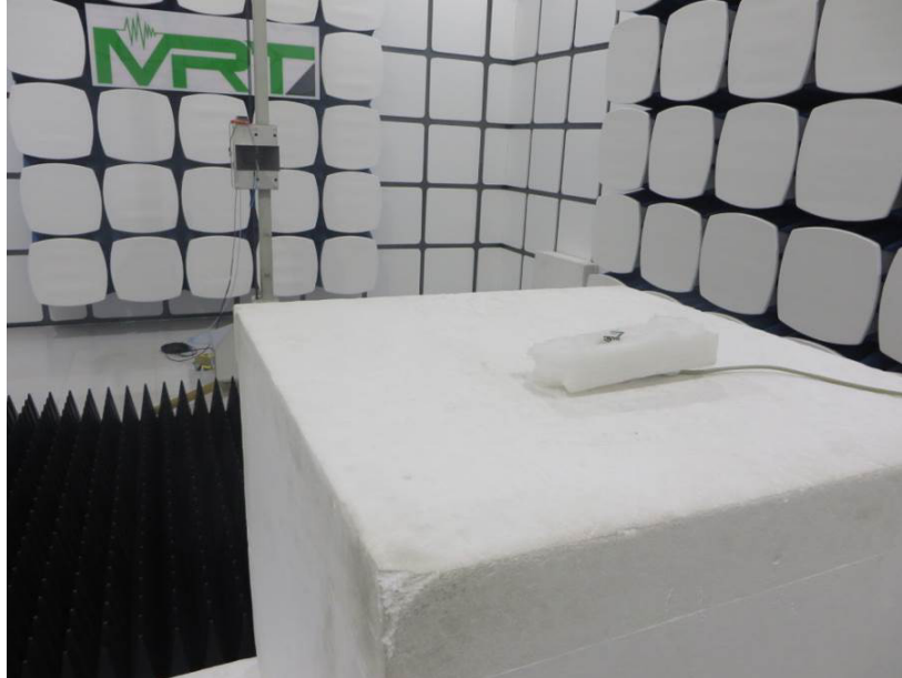
Photograph 3: Set-up for Radiated Test above 1GHz
