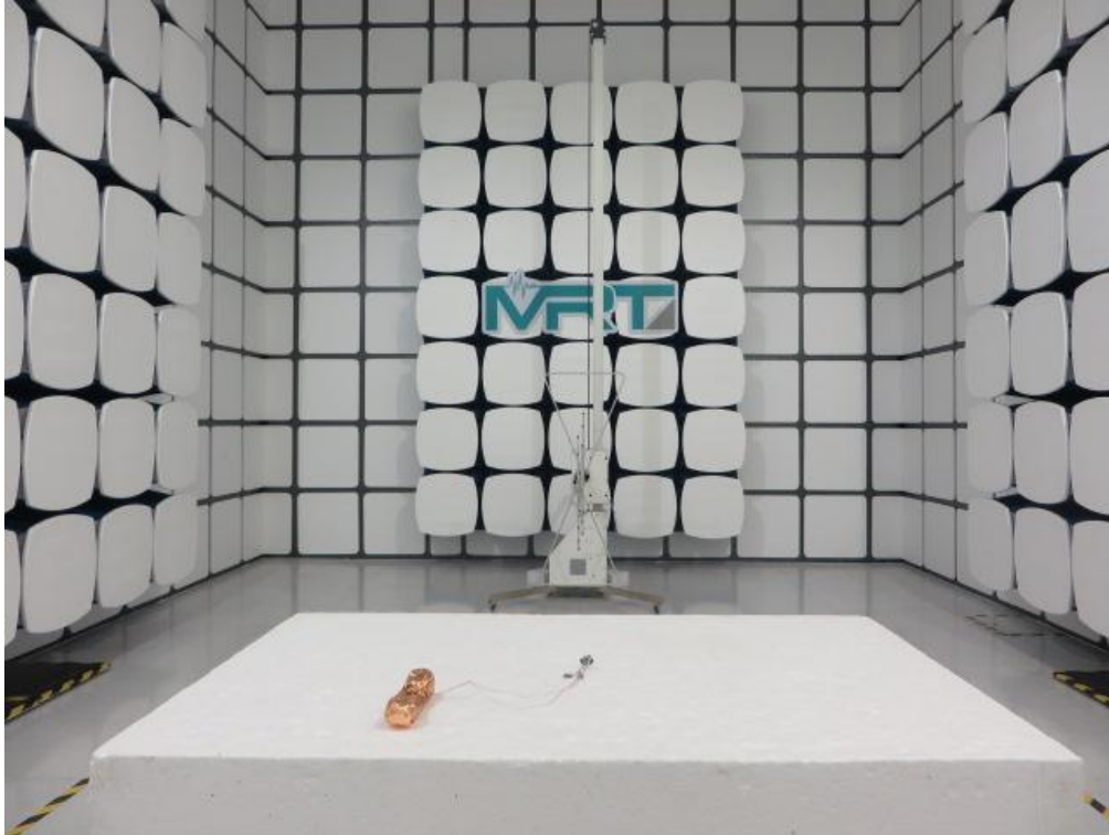
Photograph 2: Set-up for Spurious Emissions below 1GHz
