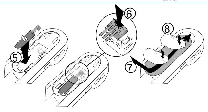
To replace the battery, with the handset turned off:
